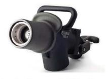
Max. Op. Pressure 5.17Bar, Max. Flow Rate 567 LPM (Options of 800 LPM, 1000 LPM), Min. Flow Rate 94.5 LPM, Inlet Port 38.1MM & 50.8 MM (1 1/2" & 2"), Weight 3.6KG
