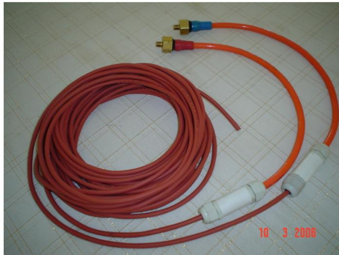
Photograph shows the 2 bar and 9 bar switches
